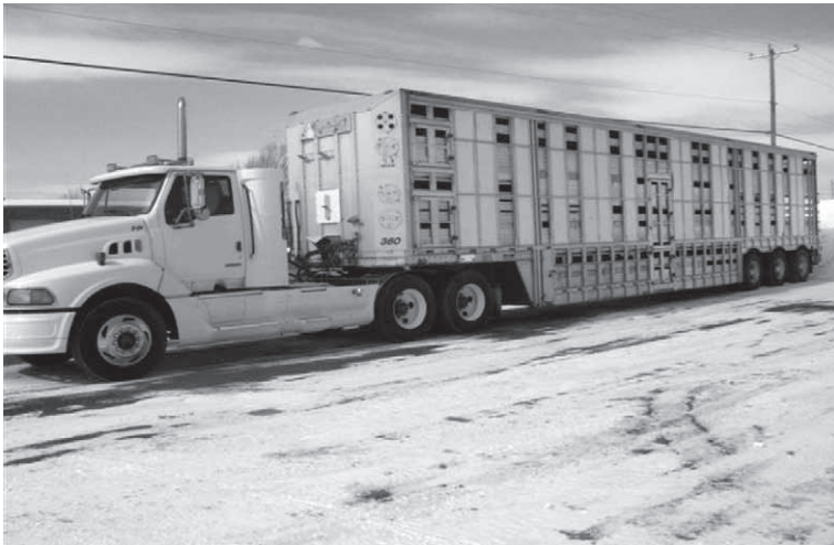
Figure 2. The pot-belly trailer is criticised for its difficulties in loading and unloading (Photo courtesy of Luigi Faucitano).
